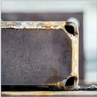
End plate venting. This is how a hollow section end plate should be cropped at all corners prior to attaching to prevent zinc and air traps.
