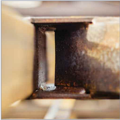
Zinc free flow. Stopping short cross beams eliminates air locks and allows free flow of zinc through the fabrication.
