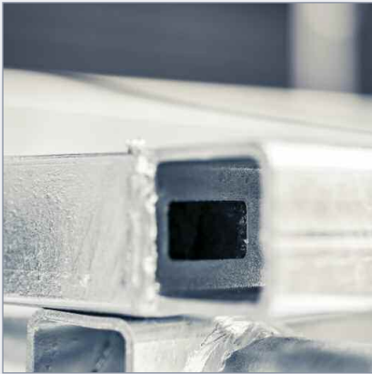
Internal venting. Before welding on the SHS leg, create internal flow by venting the main RHS member in appropriate places, as per the photo.
