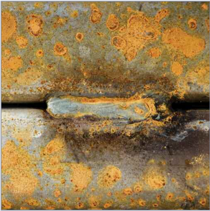
Overlapping surfaces. Leave minimum gap of 2mm between overlapping surfaces. Where seal welding is not practicable stitch welding should be used.
