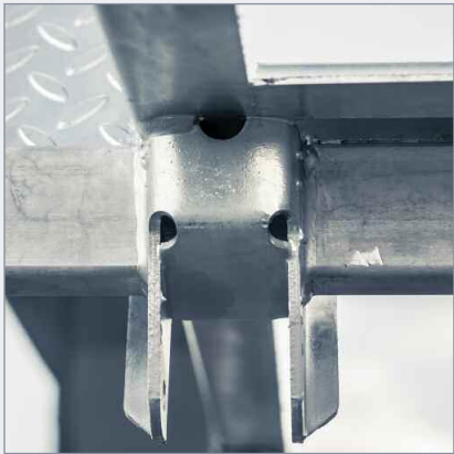
Hole stamping. Holes stamped out prior to weld assembly will make venting more than adequate.
