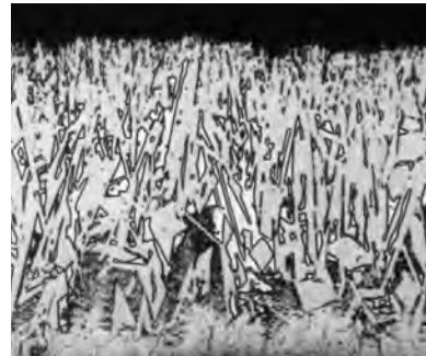
Fig. 4. Microstructure of the thick coating obtained using a silicon-rich steel.
